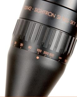
The Sightron SII 12X 42 mm is one of the company's new Big Sky series of scopes, and features an adjustable objective, ZACT-7 multicoating and the ExacTrack windage and adjustment system. Distinct markings on the target-type turrets permit fast, repeatable windage and elevation adjustments. An adjustable objective focusing ring provides parallax-free operation from 10 yds. to infinity.
